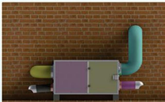
Reactivation air inlet and outlet must be located outdoors; dry air must be distributed throughout the dehumidification room; the intake air duct does not need to be connected.
